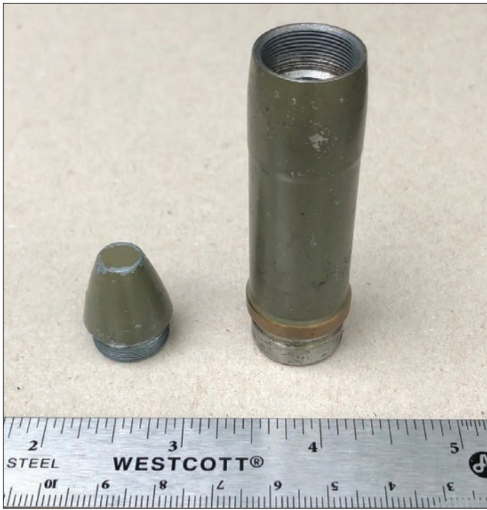
20-mm shell; machined hollow body with inert nose plug in lieu of fuse
