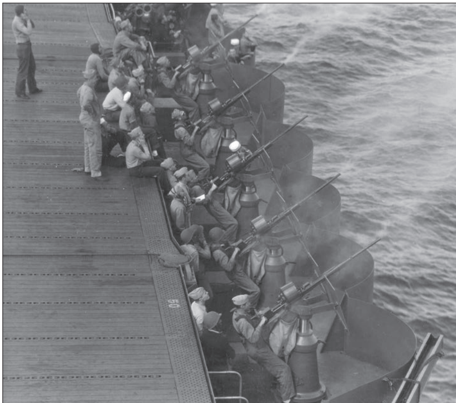
Newly installed 20-mm guns along the flight deck of aircraft carrier USS Enterprise (CV-6) firing at a target drone during gunnery practice off the Hawaiian Islands on 28 March 1942. (National Archives)
